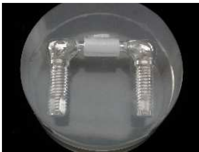
Figure 1. Bar-clip attachment system connected with two implants and embedded in a self-curing acrylic resin.
