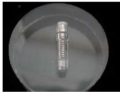
Figure 2. O'ring attachment system connected to an implant and embedded in a self-curing acrylic resin.
