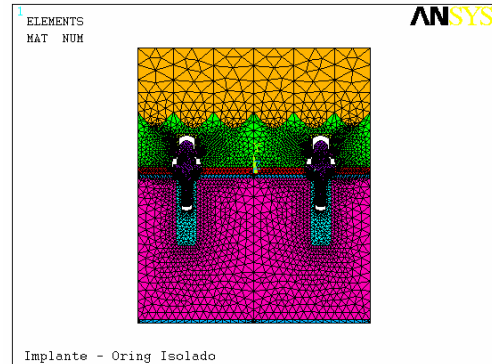
Figure 4. Finite element mesh of edentulous mandible model supporting an overdenture over two unsplinted implants with the O'ring system (IOG) (9206 elements and 19016 nodes)
