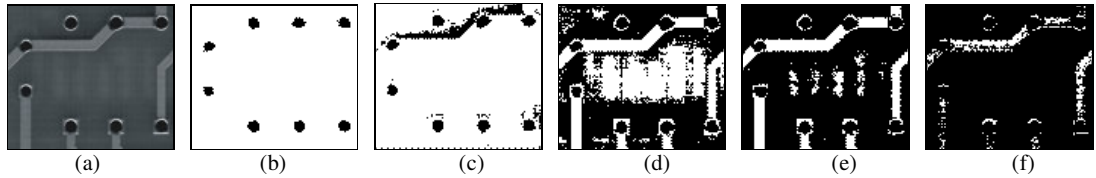
Figure 3. (a) PCB part. Threshold value equal to: (b) 4, (c) 50, (d) 70, (e) 80 and (f) 110.
