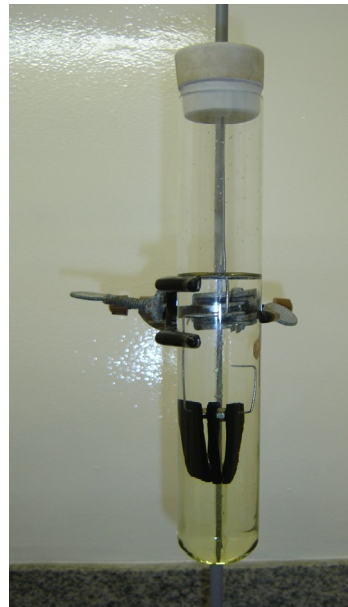
Figure 2. Submerged specimens in toluene
