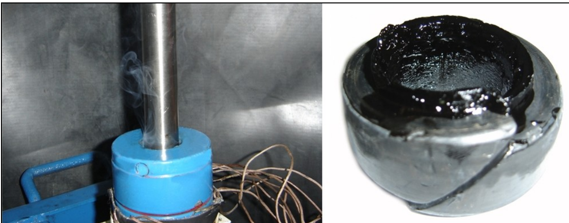
Figure 8. Smoke generated in contact surface, and fusion of the sealing surface of top seal.
