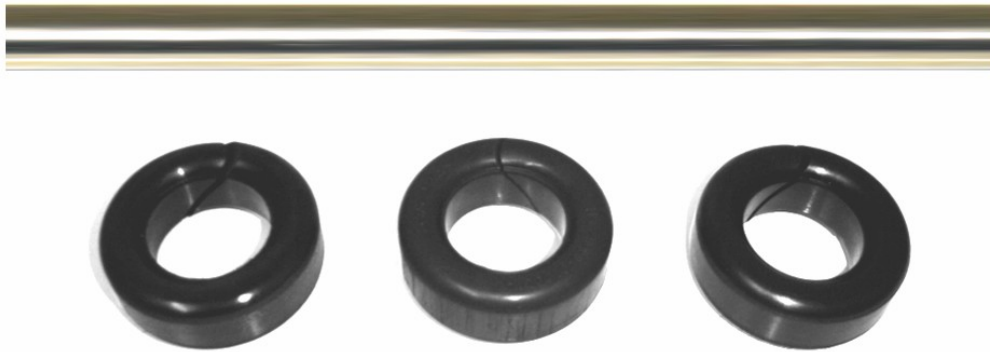
Figure 1. AISI 316 stainless steel polished rod and NBR seals
