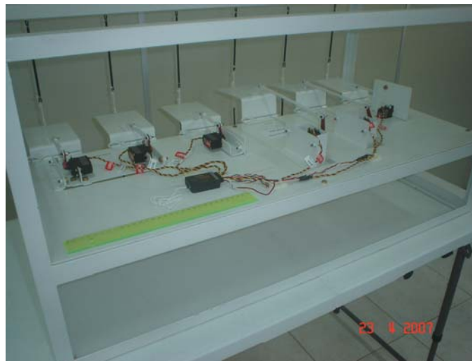
Figure 1. Servo actuator test bench
