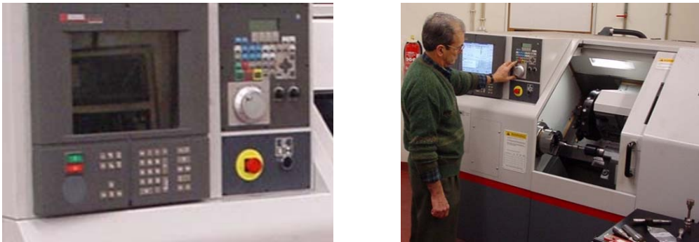
Figure 4. CNC Lathe: the man/machine interface includes user friendly elements such as a keyboard, a screen a wheel and some buttons.
