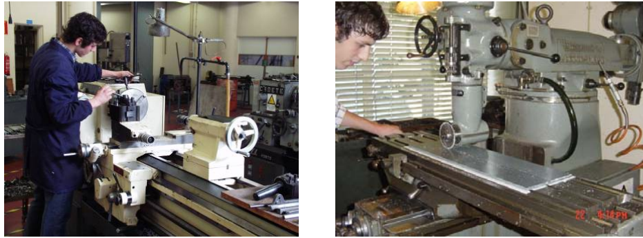
Figure 1. Conventional manufacturing operations in a lathe (left) and a in a milling machine (right); Skilled professionals are needed to handle the machines, and risk is all time present.
