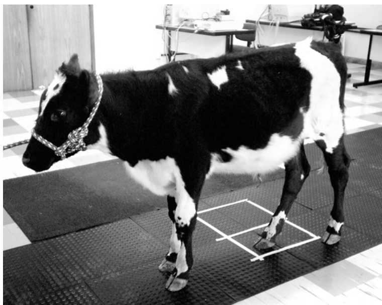
Figure 1. The calf stepping with the right hind limb over the force plate during the experiment.
