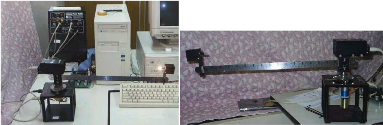
Figure 1. (a) The FLECAM Quanser System (b) Hub, camera and flexible beam
