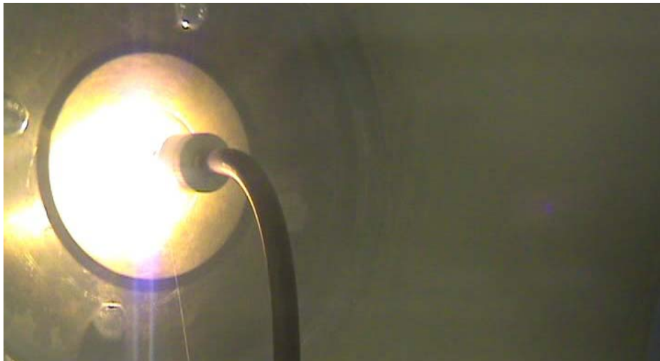
Figure 7. The view of calorimeter being streamed with hypersonic plasma jet
