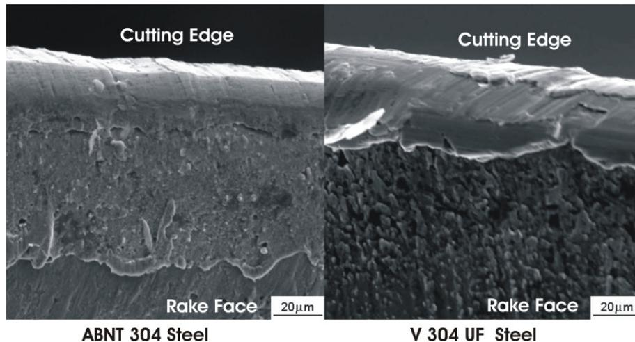
Figure 6 Adherent layer that covers the drill main cutting edge.
