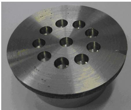
Figure 1. Workpiece after the measuring the feed force and torque.
