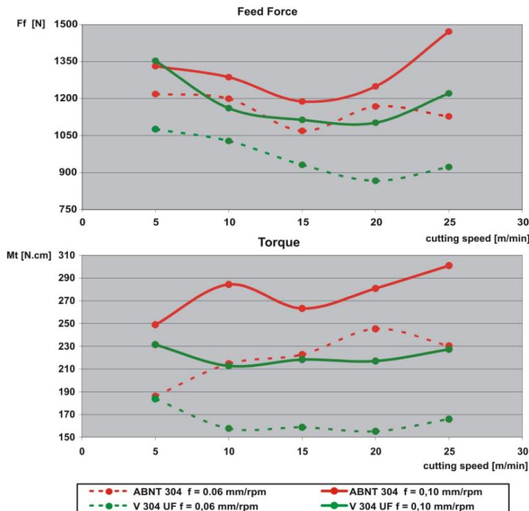
Figure 5 – Differences in feed force and torque at five cutting speeds.
