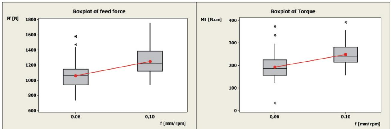
Figure 3 – Differences in feed force and torque with two drill feed rates.
