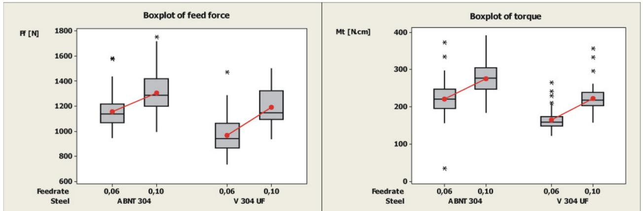
Figure 4 – Differences in feed force and torque with two feed rate drills and two austenitic stainless steels.
