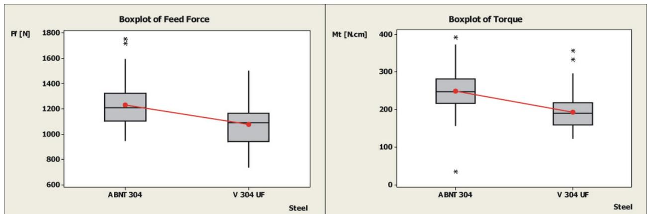
Figure 2 – Differences in feed force and torque with two austenitic stainless steels.
