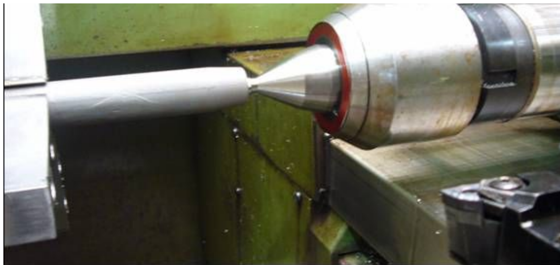
Figure 7 – Experiment assemblage for the external cylindrical cutting operation.
