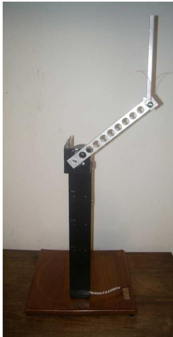
Figure 1. Physical implementation of a rotary inverted pendulum built at LARA in UnB.
