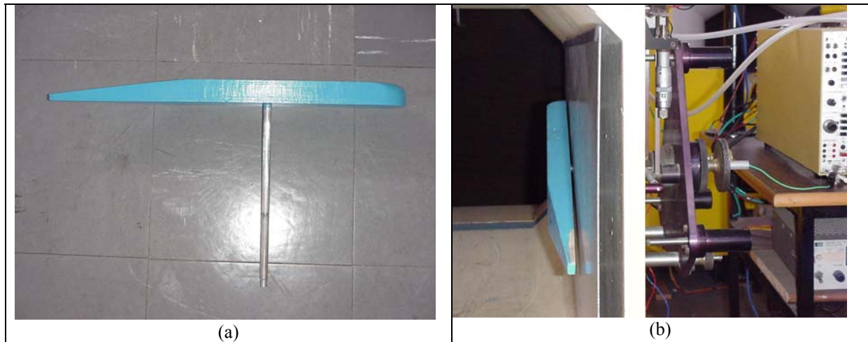
Figure 3: (a) Half fuselage model and its metal axis and (b) rear view of the model inside the wind tunnel test section.
