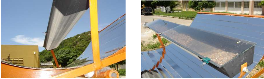
Figure 2.3. Absorber gutter in the system focus
