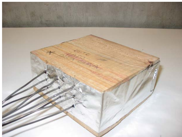
Figure 3. Configuration of thermocouples inside the slabs.
