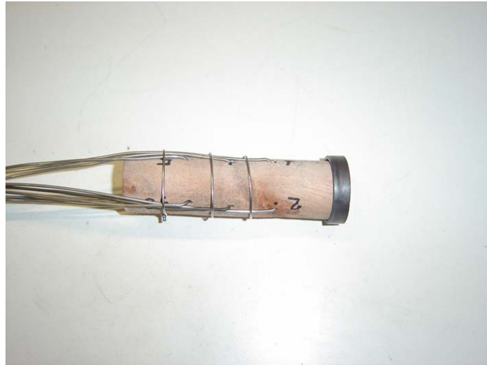
Figure 2. Configuration of thermocouples inside the cylinders.
