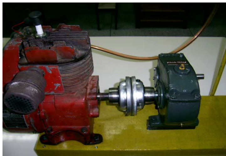
Figure 3 – Test rig built with Montgomery engine and Cestari Reducer brand
