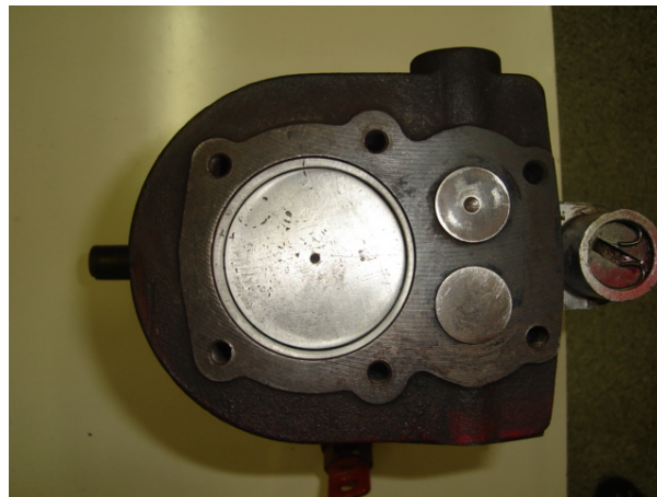
Figure 6 – Piston head of Montgomery engine after the test
