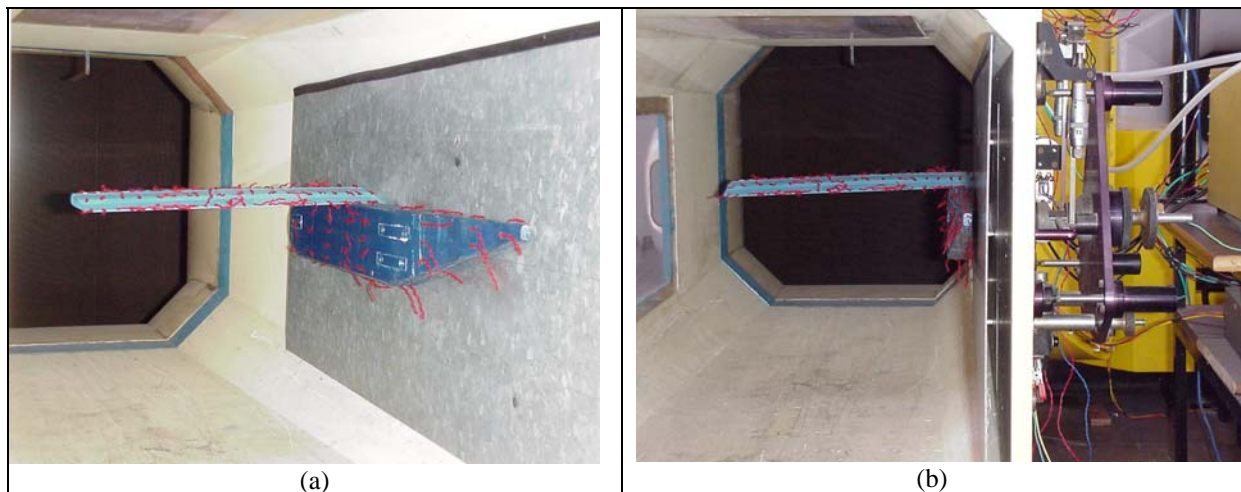
Figure 3: (a) Wing-fuselage half model assembled at the wind tunnel (b) rear view of the model inside the wind tunnel test section.
