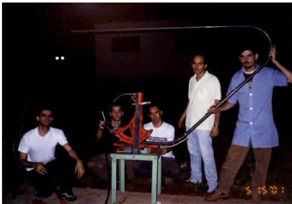
Figure 1. Construction of the vehicle. On the left students curving a tube for the structure, on the right the mounted structure.
