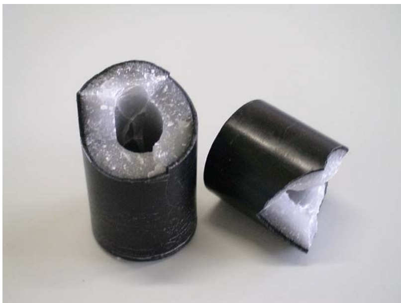
Figure 7 - Paraffin grain prepared without dispersant and tested in low temperature.
