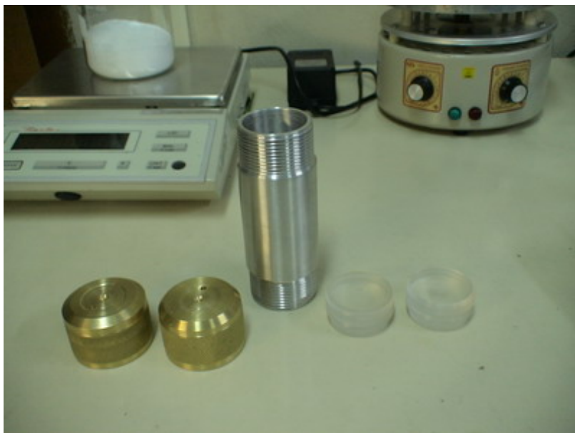
Figure 1: Brass covers with screws, aluminum tube and PMMA covers.
