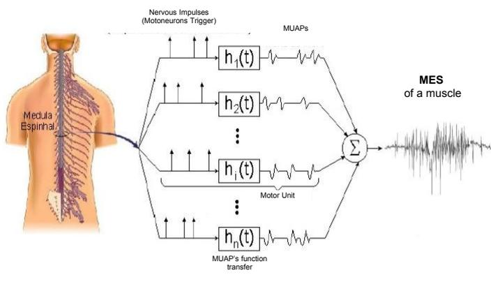
Figure 2. Schematic representation of MES composition
