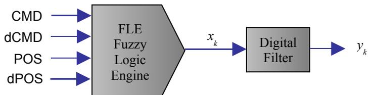
Figure 10. Diagrammatic representation of smoothing process of output signal
