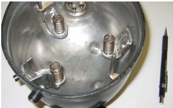
Figure 1-a. Cylindrical helical suspension springs in the compressor.
