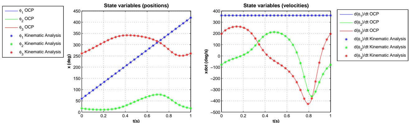
Figure 2. Comparison of state variables trajectories for CASE 1 with kinematic analysis of 4-bar mechanism.
