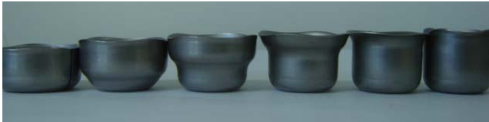
Figure 4. Stages of redrawing operation.
