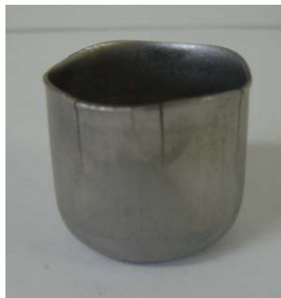
Figure 2. Delayed Cracking Phenomenon in A stainless steel for \text{LDR-DC}=2.15 .
