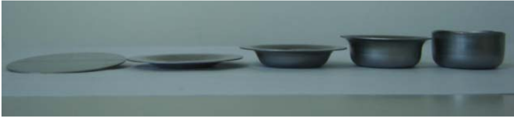
Figure 3. Stages of deep drawing operation.
