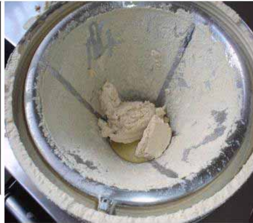
Figure 12. Soya protein residues in the filter.
