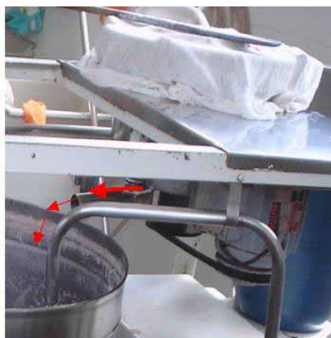
Figure 10. Filtering output to tank 2.
