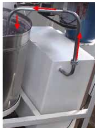
Figure 14. Outlet of product to tank 2.
