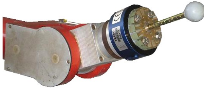
Figure 6. Force sensor and end-effector.
