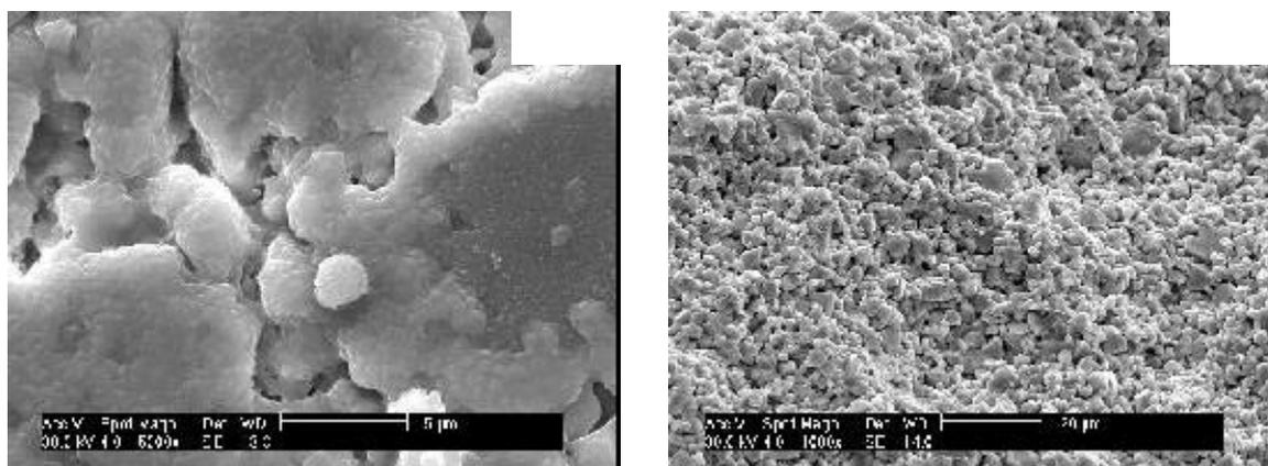
Fig. 4 SEM micrograph of  $Ba_2NiWO_6$  ceramics sintered at 1300°C, (a) polished surface (5000x); (b) fracture surface (1000x)
