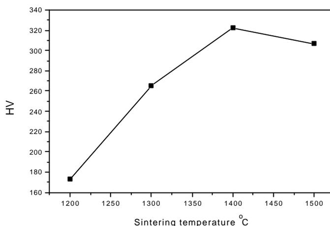
Fig. 7 Variation of Vicker's hardness values as a function of sintering temperature in sintered  $Ba_2NiWO_6$  ceramics
