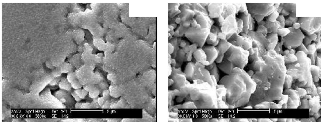
Fig. 3 SEM micrograph of  $Ba_2NiWO_6$  ceramics sintered at 1200°C, (a) polished surface (5000x); (b) fracture surface (1000x)
