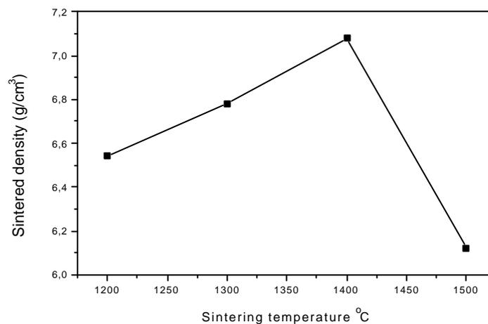
Fig. 6 Variation of sintered density as a function of sintering temperature
