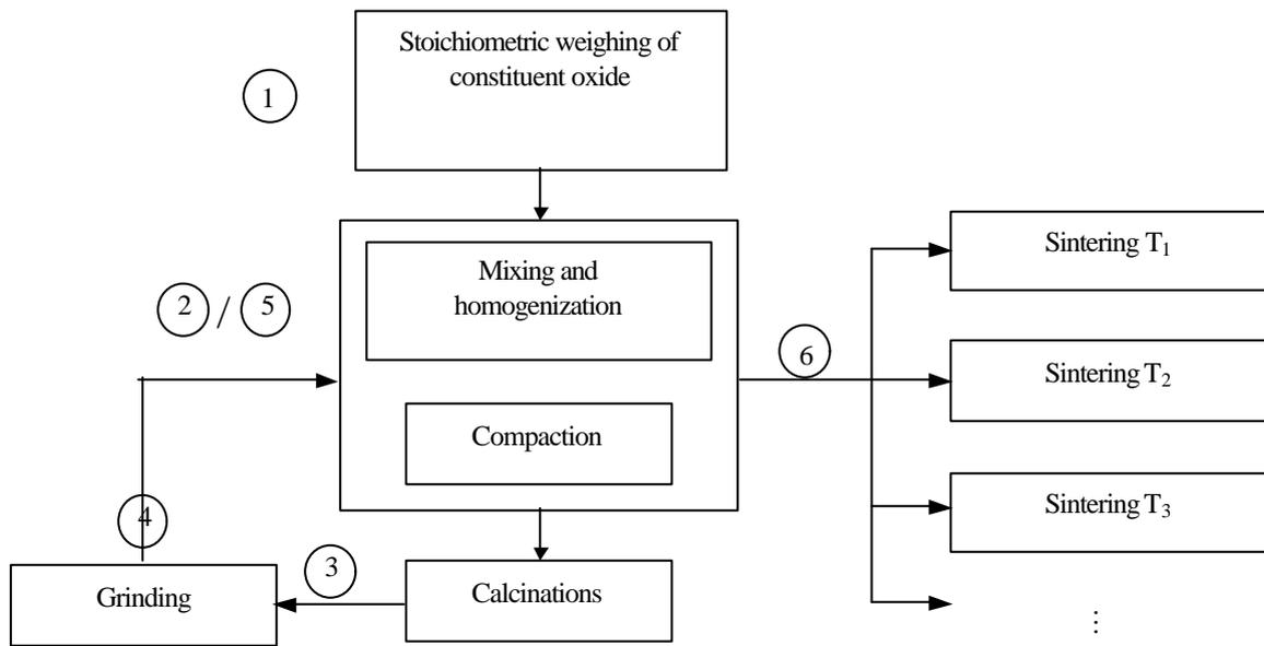
Figure 1 Flow chart for preparation and sintering of  $\text{Ba}_2\text{NiWO}_6$
