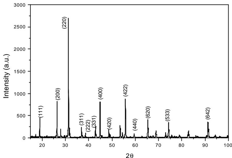
Fig. 1: Powder X-ray diffraction patterns of  $Ba_2NiWO_6$  ceramic, sintered at  $1200^\circ C$
