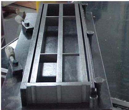
Figure 1. Mold used in the production of the polymer concrete beams.
