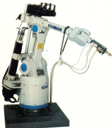
Figure 3. Flame thermal spray robot.
