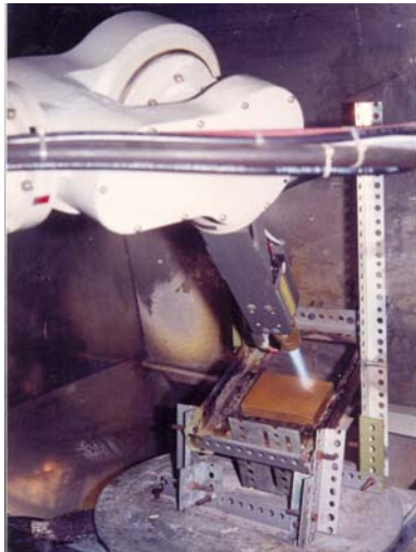
Figure 5. Robotic oxyacetylene preheating (spray angle 65°).
