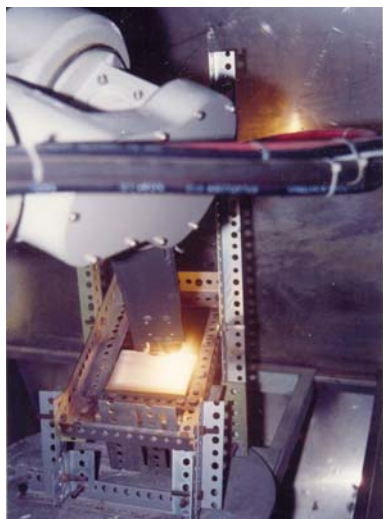
Figure 8. Robotic spraying of the zirconia coating (spray angle 65°).
