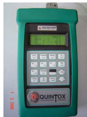
Figure 6. Control unit of the analyzer.
