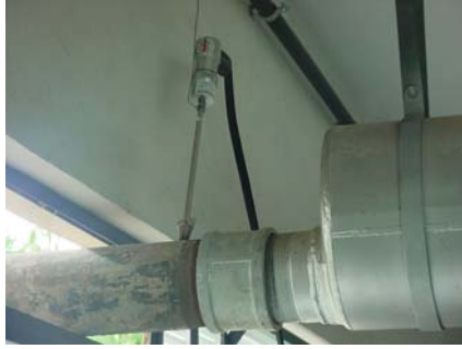
Figure 7. Probe of the gas analyzer
