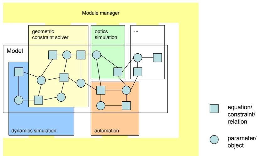
Figure 3. Specialized calculation modules/solvers handle parts of the model. In some cases a model part can be calculated by more than one module. Then, the module manager decides which module handles this part depending on the task.
