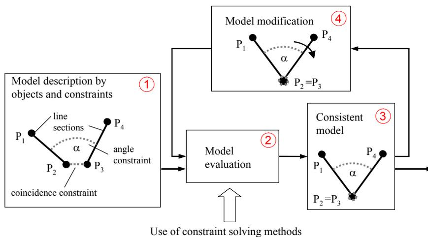
Figure 1. Calculation cycle in constraint based modeling.
