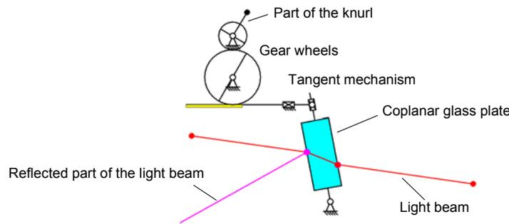
Figure 7. Solution principle of a micrometer modeled in the design system
