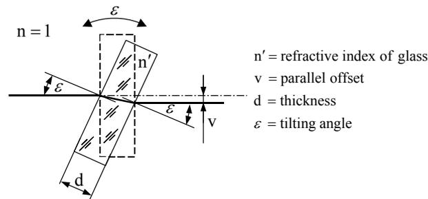
Figure 5. Parallel offset of the main beam by a coplanar glass plate
