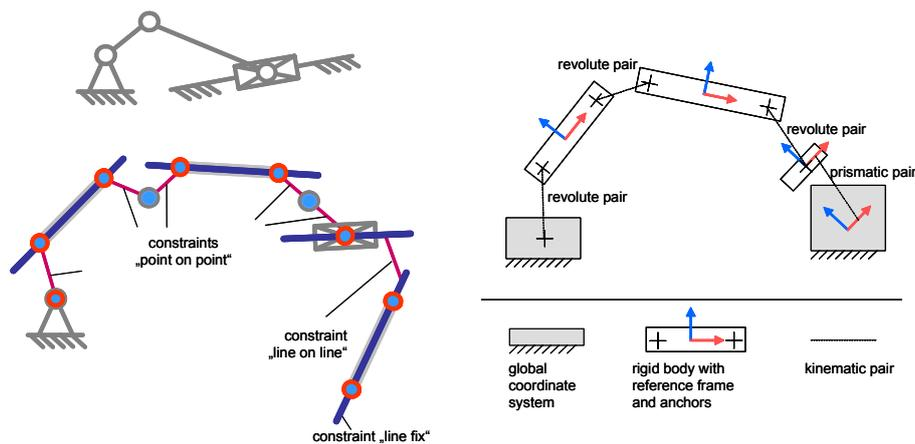
Figure 4. Transformation of the abstract model description (upper left) of a slider crank into specific representation for a geometric constraint solver (left) and for multi-body simulation (right)
