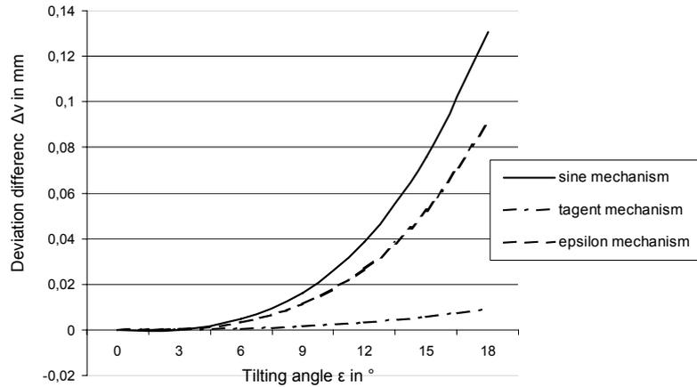
Figure 6. Difference  $\Delta v$  between  $v_{\text{approx}}$  of the approximations from Table 1 and  $v$  of the original transfer function (Eq. 1) for different tilting angles  $\epsilon$  (assumption: refraction index  $n=1,519$ ; thickness of the glass plate 22,44mm).
