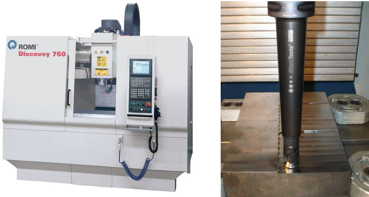
Figure 2 – ROMI Discovery 760 machining centre and anti-vibration tool.
