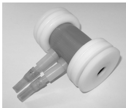
Figure 2. Cell used in the corrosion fatigue tests in the aggressive environment.
