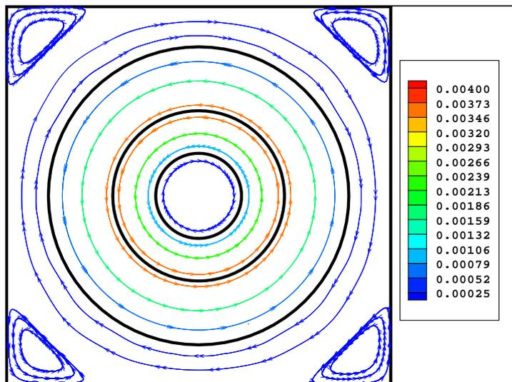
Figure 5. Ring region flow of three rotating concentric cylinders. The case in which the middle cylinder rotates counter-clockwise. Streamlines in function of the velocity norm (black lines represent the circular concentric cylinders).
