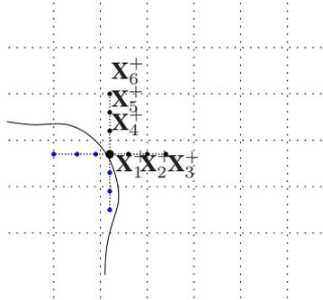
Figure 3. Additional points  $\mathbf{X}_1^+, \dots, \mathbf{X}_6^+$  e  $\mathbf{X}_1^-, \dots, \mathbf{X}_6^-$  used on determination process of force term components (4) and (5), respectively.
