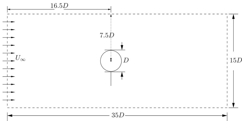
Figure 6. Geometry for flow passing a stationary cylinder.
