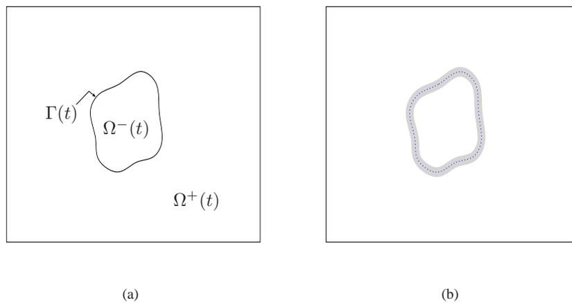
Figure 1. Immersed Boundary Method: (a) geometrical configuration of fluid-stuture interaction; (b) force field on the equations of fluid imposing structure presence.
