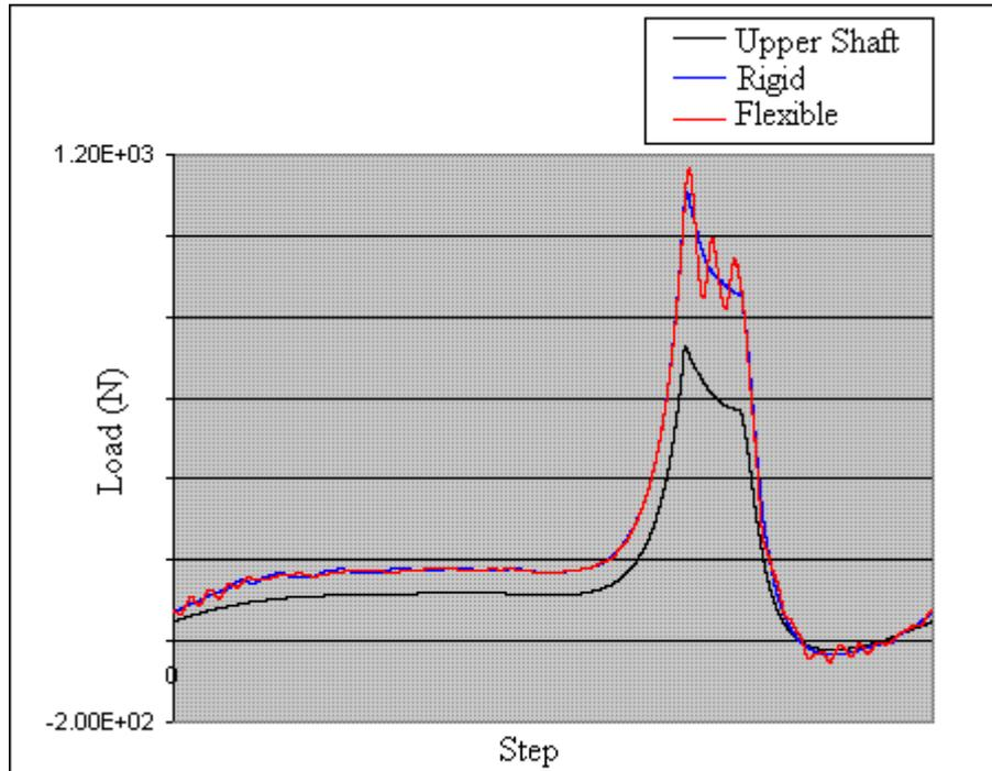
Figure 6. Rigid and Flexible Shaft considering  $k = 1 \cdot 10^8$ ;  $c = 1 \cdot 10^5$ ;  $n = 5$ ;  $m = 1$ .
