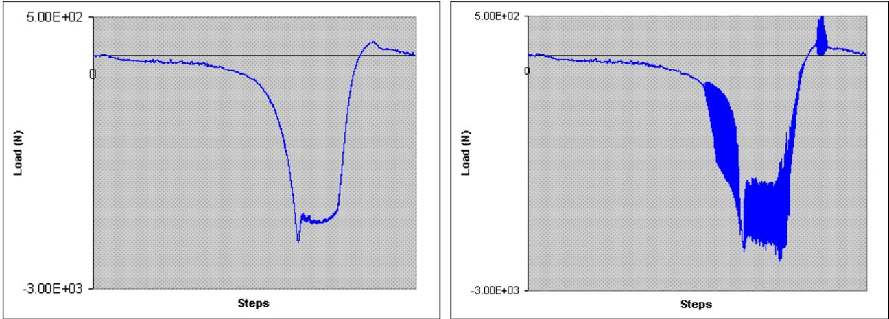
Figure 2. Two loads graphics of the upper bearing. The left system is stable and the right one unstable.
