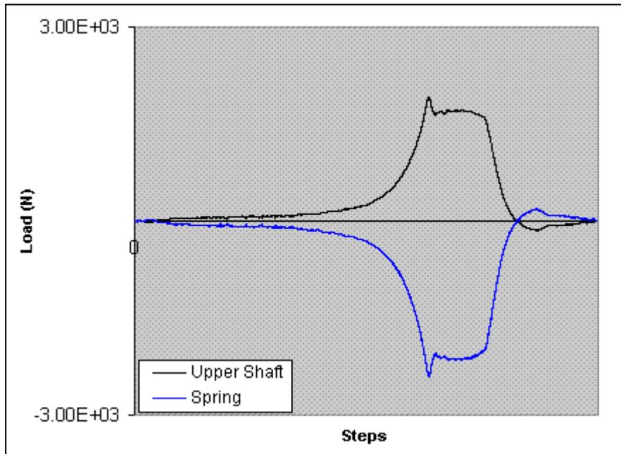
Figure 4. Comparison between upper shaft load and the oil film load.
