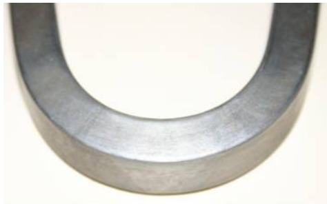
Figure 14. Bending test – ASME IX.
