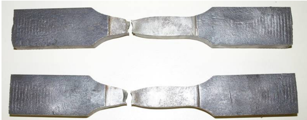
Figure 13. Tension test – ASME IX.
