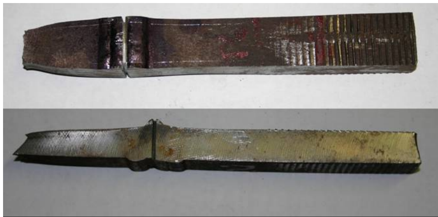
Figure 16. Result of the nick break – ASME IX.
