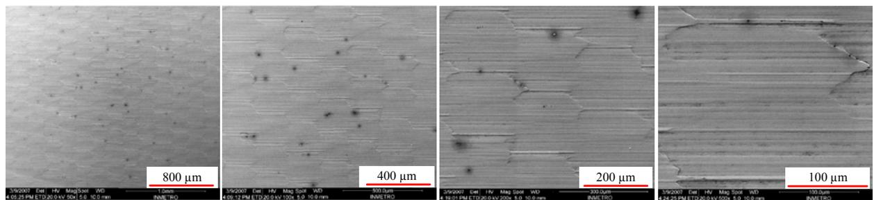
Figure 7. Images of SEM (secondary electrons), strategy VD with magnification of 50x, 100x, 200x and 500x
