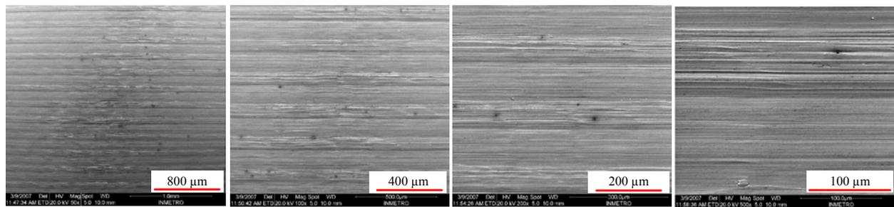
Figure 9. Images of SEM (secondary electrons), strategy HD with magnification of 50x, 100x, 200x and 500x
