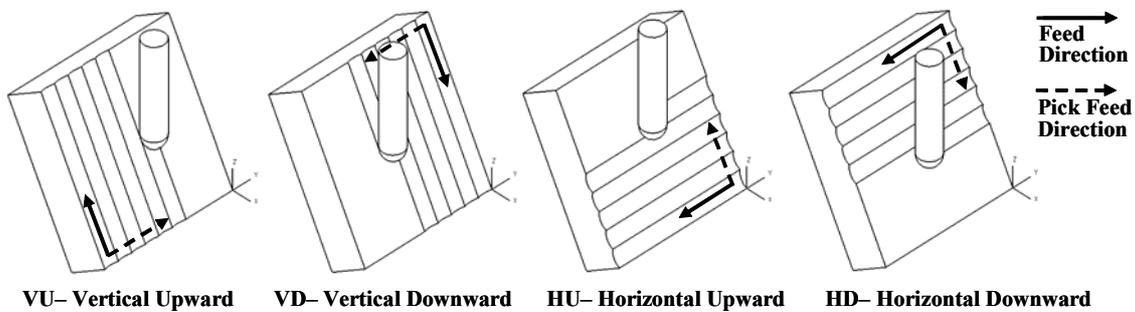
Figure 1. Considered cutter path orientations
