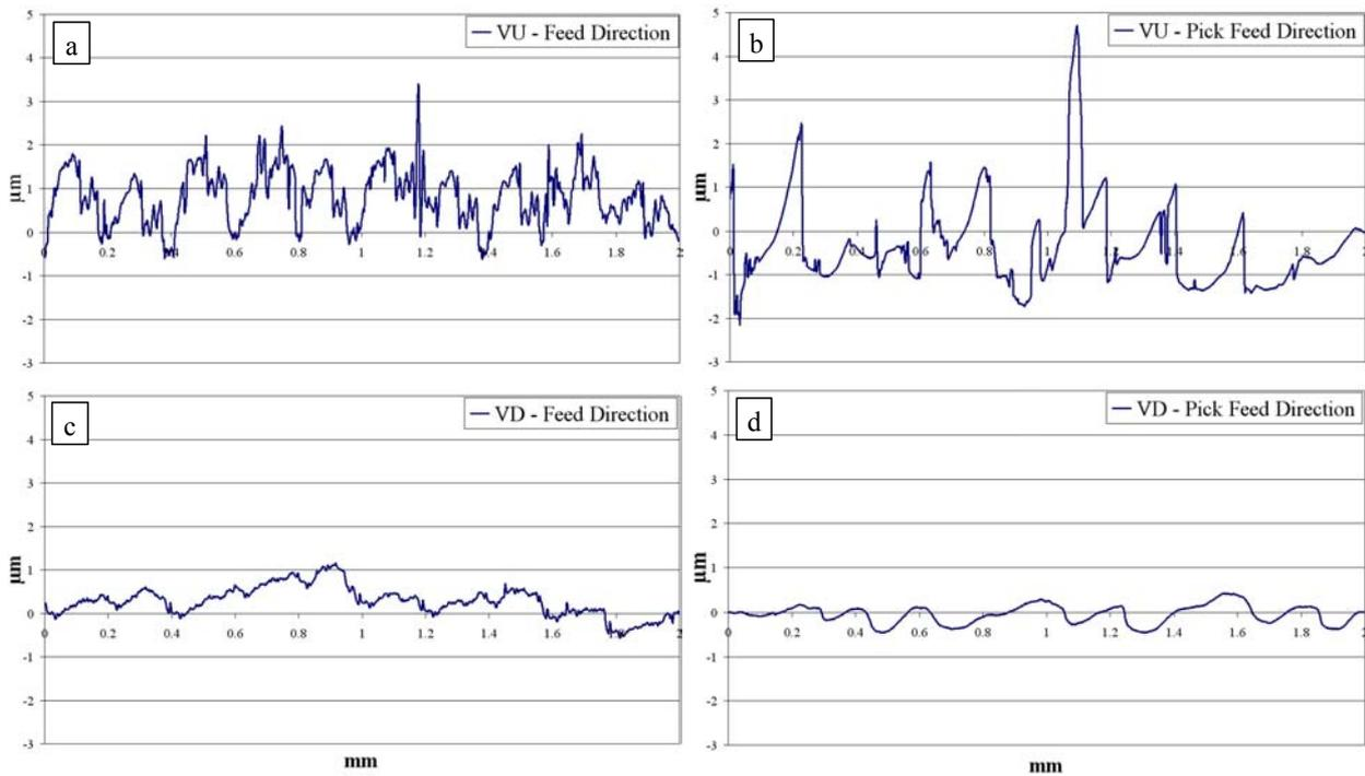
Figure 4. Roughness graphics for vertical upward (4a, 4b) and vertical downward (4c, 4d)
