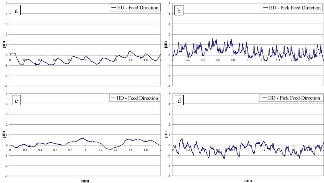
Figure 5. Roughness graphics for horizontal upward (5a, 5b) and horizontal downward (5c, 5d)
