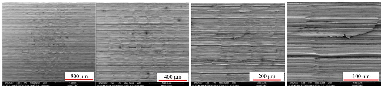
Figure 8. Images of SEM (secondary electrons), strategy HU with magnification of 50x, 100x, 200x and 500x
