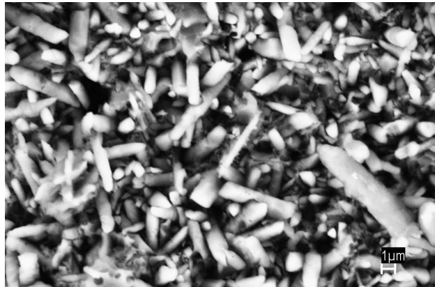
Fig 3 – SEM micrograph of polished and etched surface of substrate.
