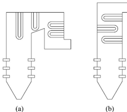
Figure 2. Two configurations for the supercritical boiler to date: a) two-pass design and b) tower design.
