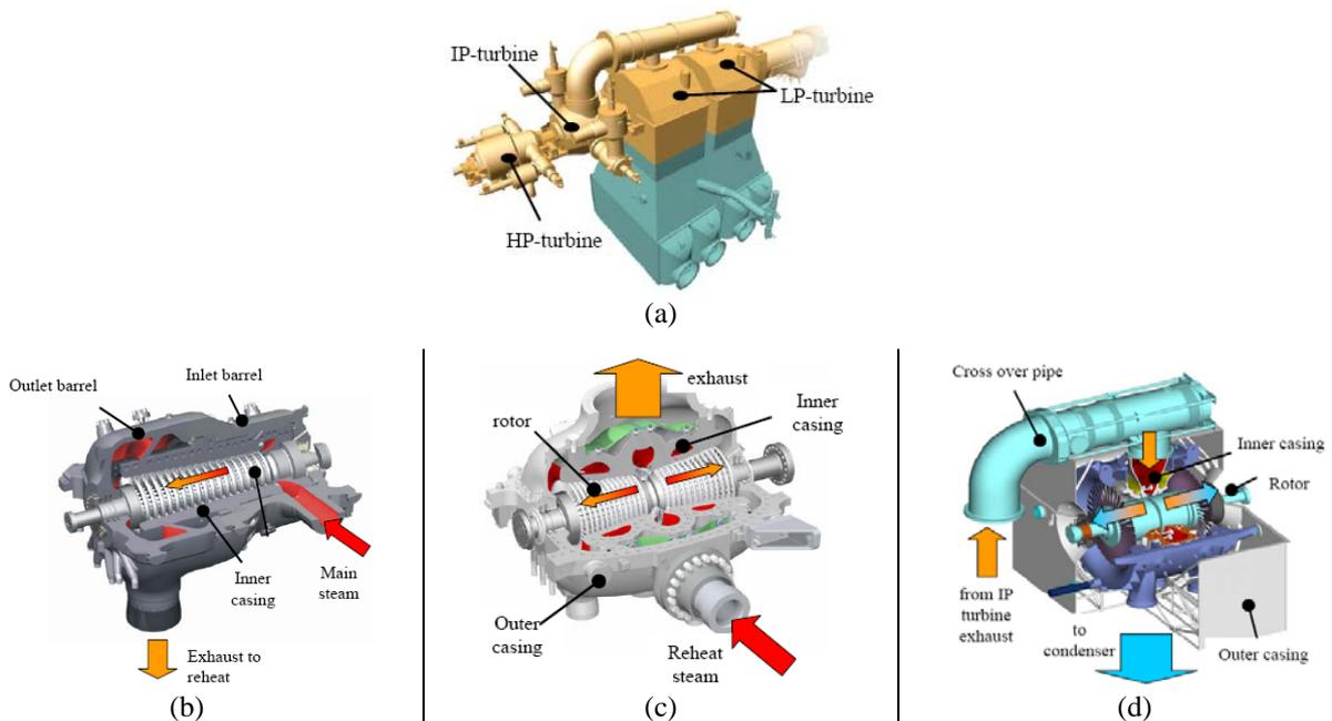
Figure 3. (a) 600-1000MW-class turboset. (b) Barrel-type high pressure turbine (HP). (c) Intermediate pressure turbine (IP). Low pressure turbine (LP) (Rosenkranz and Wichtmann, 2005).
