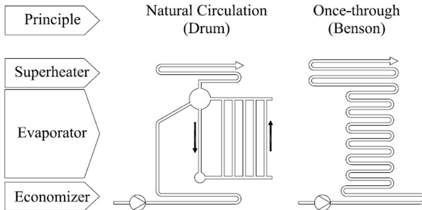
Figure 1 – Water/Steam Path in Drum Boilers and Once-through Boilers.
