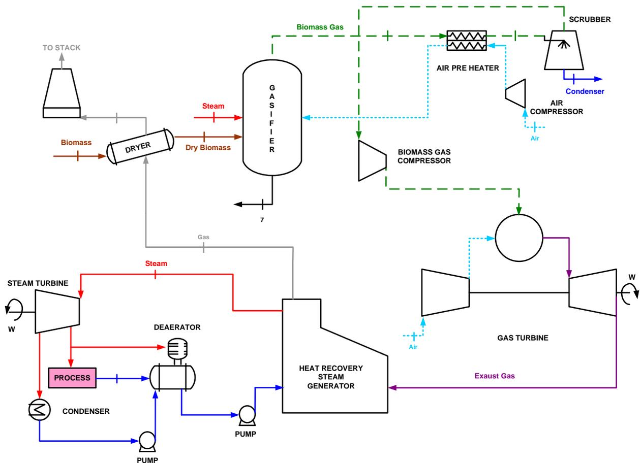
Figure 5 - Schematic representation of the BIGCC
