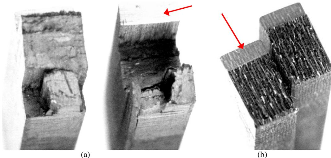
Figure 06 – Fracture surfaces of C-Ep laminates tested under identical conditions: (a) Tape, and (b) Fabric array of reinforcing carbon fibers. Note the flat topology in (b), signaling a very low capacity of energy absorption during the specimen rupture.
