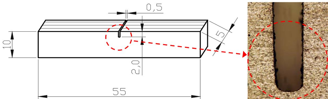
Figure 03 – Charpy impact specimen geometry according to the ASTM D5045 standard [15] (sizes in mm). The approximately 0.25 mm root radius of a notch in a TiGr specimen is shown in detail.
