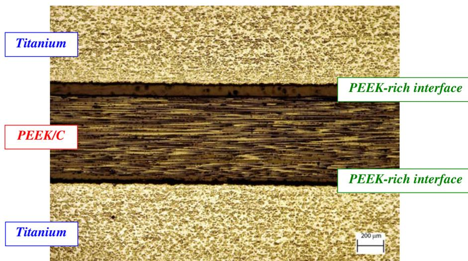
Figure 01 – Longitudinal cross-section of TiGr laminate in which its constituents are identified.
