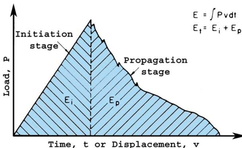
Figure 04 – The two stages of the instrumented Charpy impact test curve [9].
