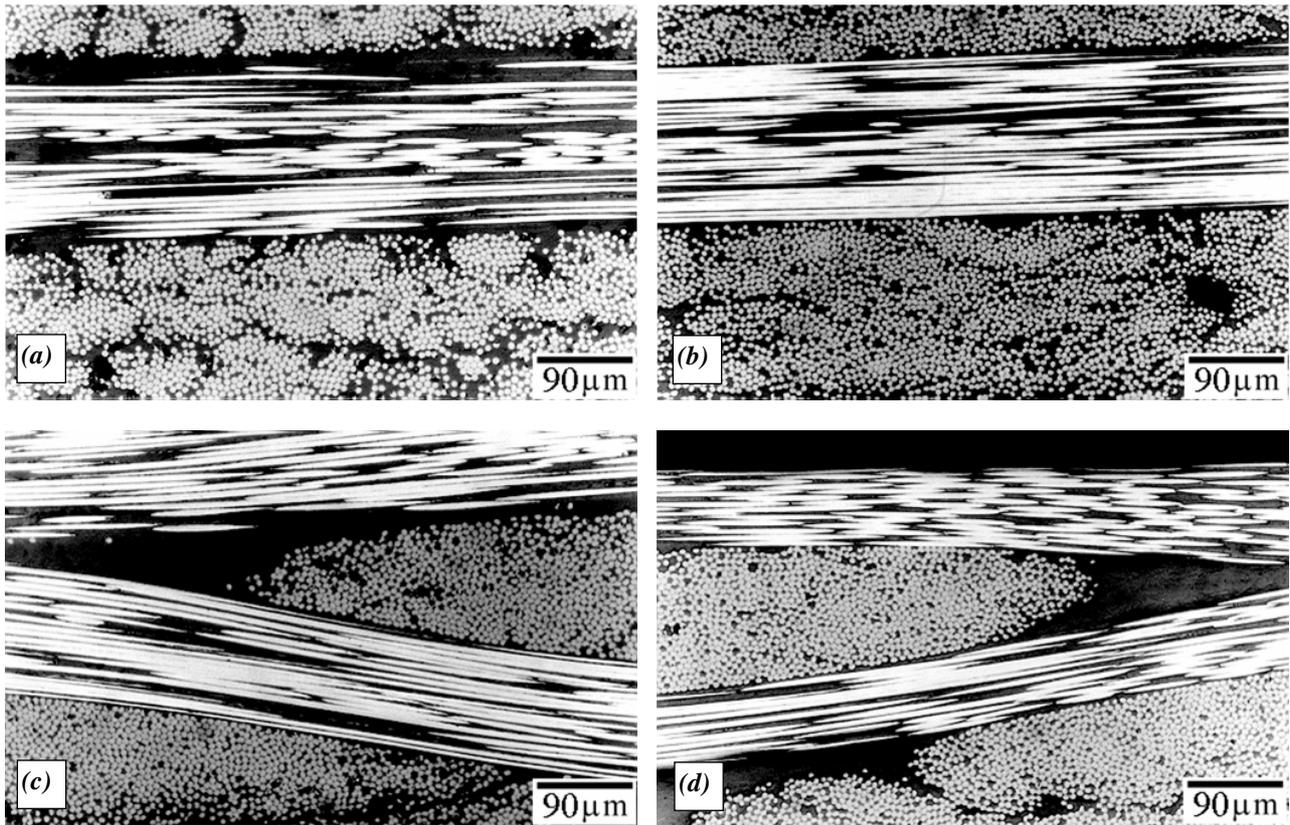
Figure 02 – Microstructure of the C-Ep laminates: (a) TP120, (b) TP180, (c) FA120, and (d) FA180.
