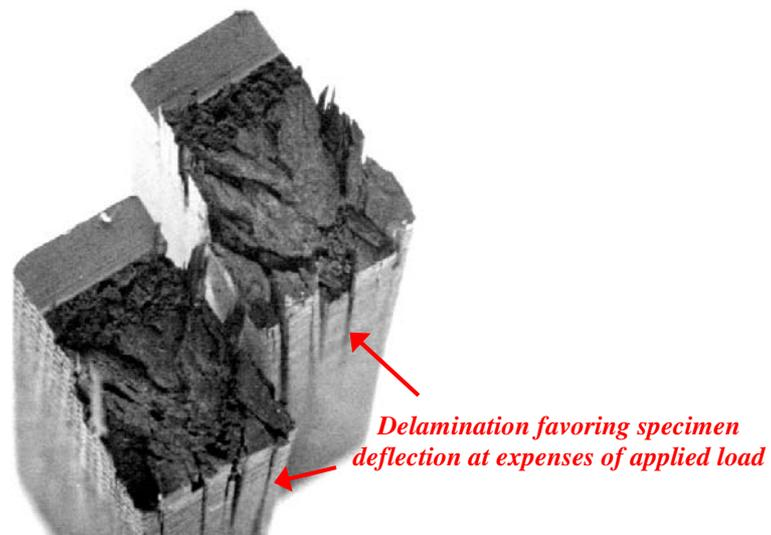
Figure 08 – Trespiece halves of TP180 laminate tested at  $-70^{\circ}\text{C}$ , where numerous delamination planes were induced by differential thermal contraction in-between simultaneous composite plies.
