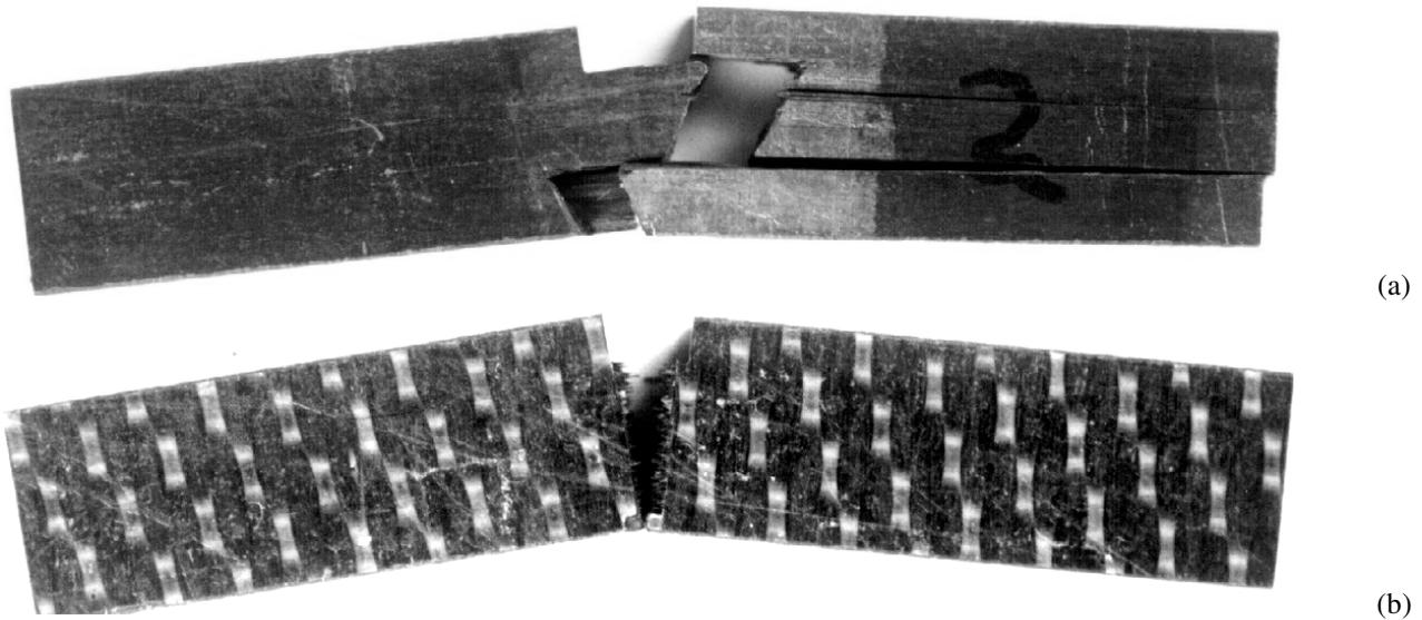
Figure 07 – Laminates TP120 (a) and TC120 (b) tested under identical conditions and exhibiting quite different cracking patterns.
