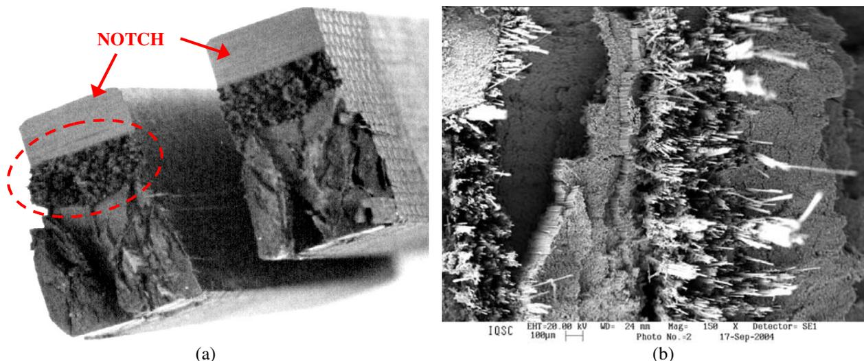
Figure 09 – Fracture surfaces of TP180 laminate tested at 100°C: (a) General view; (b) Localized view by using scanning electronic microscopy techniques.
