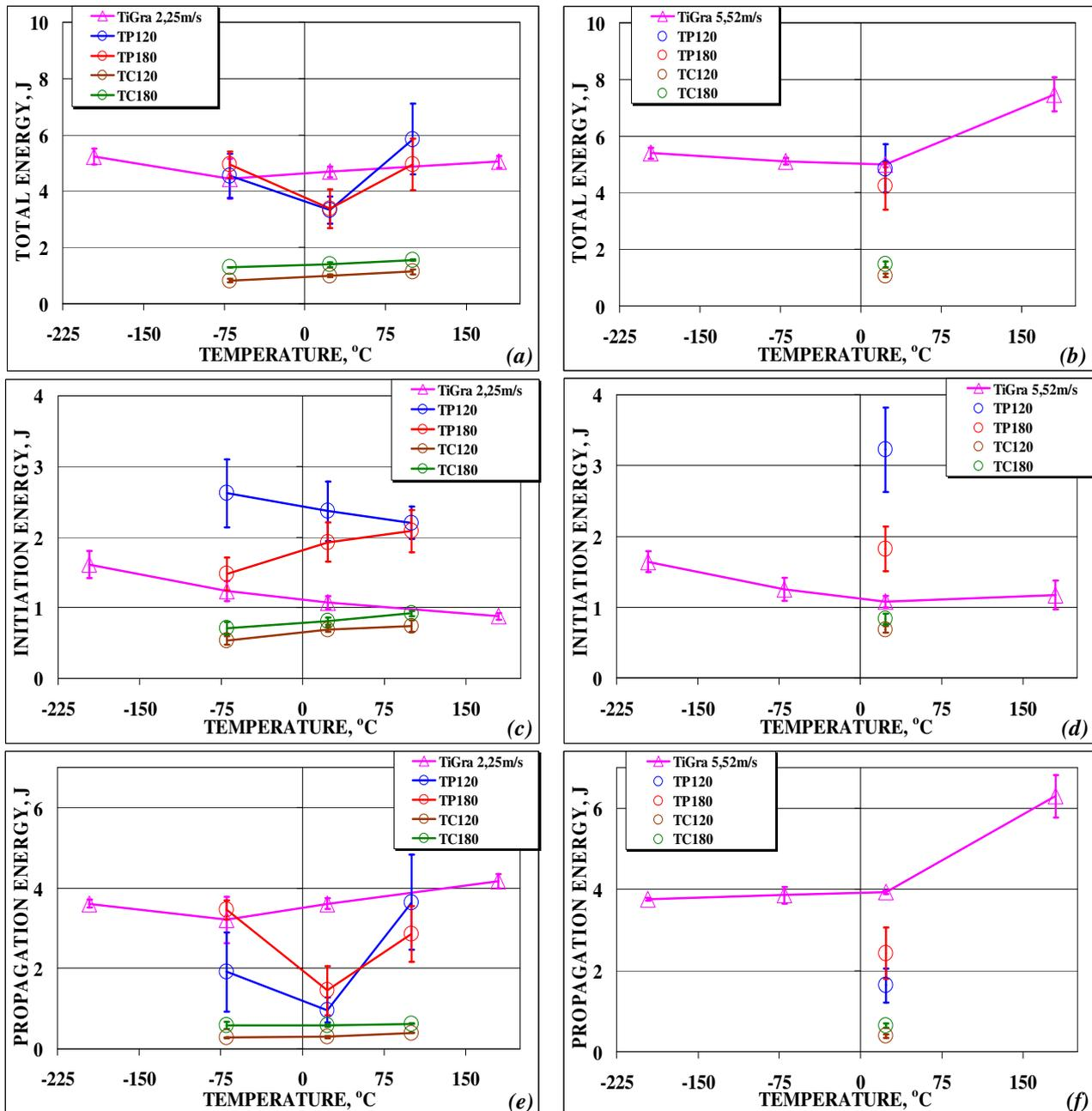
Figure 05 – Test results at different temperatures and applied loading rates for the studied laminates: (a) and (b) Total absorbed energy -  $E_t$ ; (c) and (d) Initiation energy -  $E_i$ ; (e) and (f) Propagation energy -  $E_p$ .
