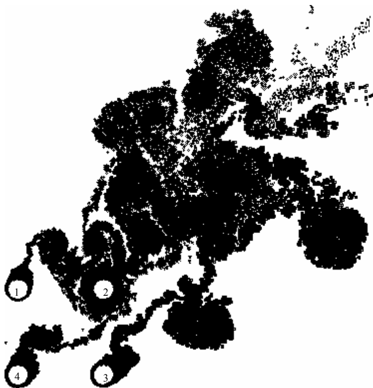
Figure 2. Position of the wakes vortices at t=60 for l/b=4 , \alpha=45^\circ , Re=1.3 \times 10^4 , \epsilon=\sigma_0=0.03b , \Delta t=0.05 , M=50 .
