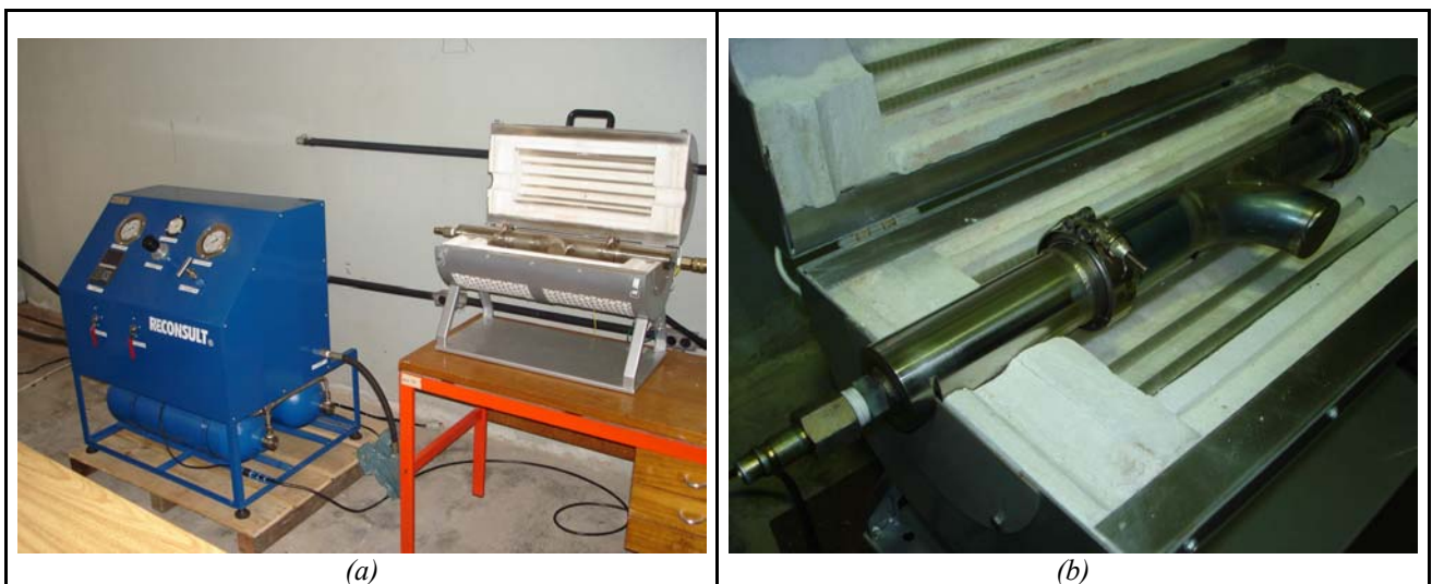
Figure 4. Pneumatic workbench: (a) general view; (b) detail of the test piece inserted in furnace
