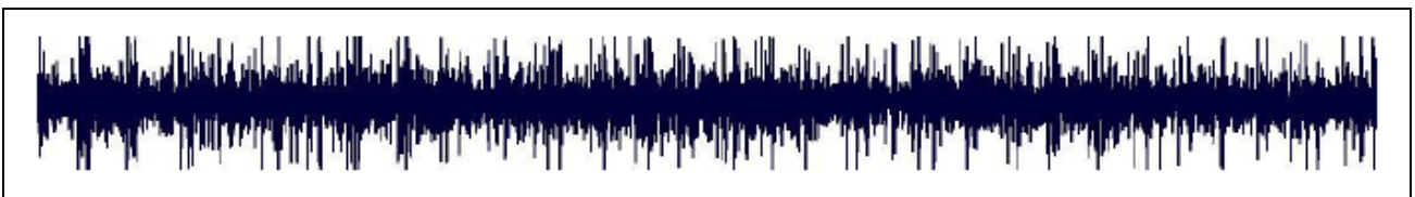
Figure 6. Metallic transference in globular mode displayed in power (volts at input) versus time
