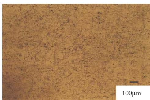
Figure 5 - Microstructure of the sheet 4.0 mm, alloy A5052, in the annealed state.
