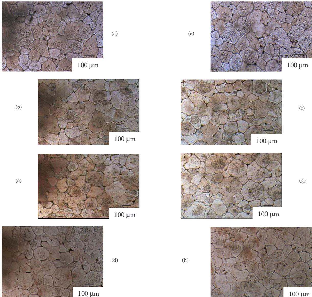
Figure 7 – Typical microstructures of a A5052 aluminium alloy sheet, 0.8 mm thickness, treated at 634°C during 10 minutes, in different regions. Sample with dimensions 200 x 200 mm, (a-h) regions of analysis.
