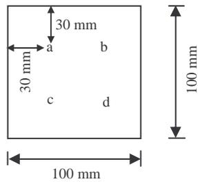
Figure 11 - Representative scheme of the regions of analysis of the thixocast sheet's microstructures, dimensions 100 x 100 mm.
