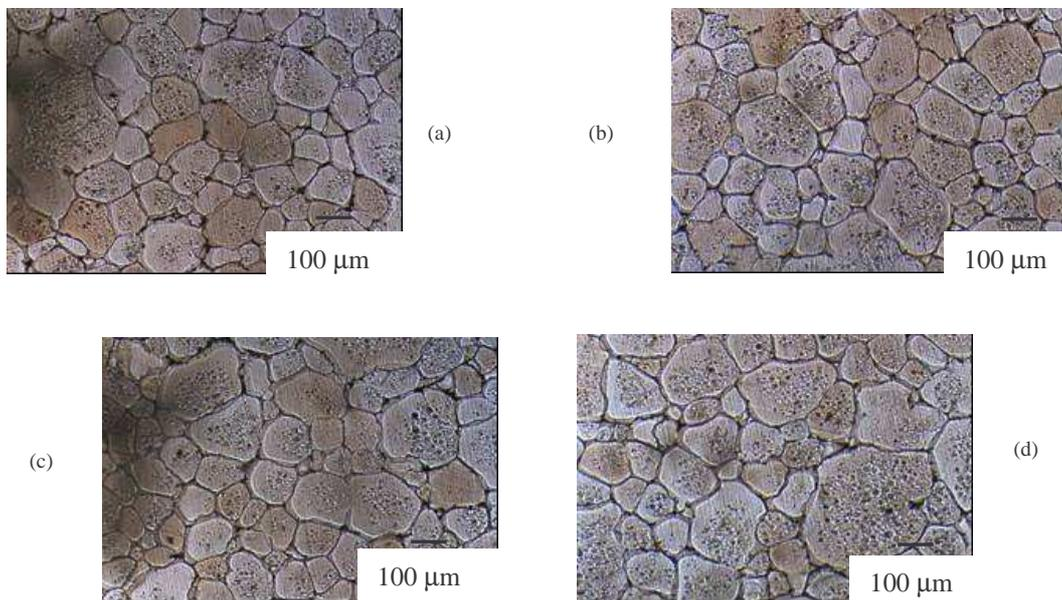
Figure 12 – Typical microstructures of a A5052 aluminium alloy sheet, 4.0 mm thickness, treated at 630°C during 10 minutes, in different regions. Sample with dimensions 100 x 100 mm, (a-d) regions of analysis.
