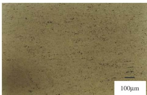
Figure 3 – Microstructure of the sheet 0.8 mm, alloy A5052, in the rolled state.
