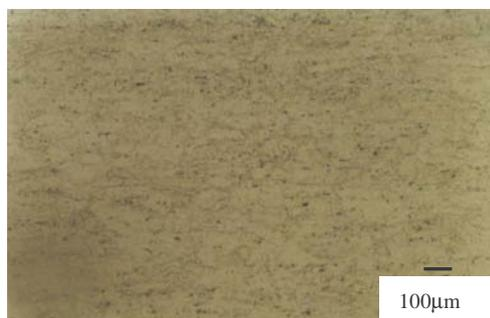
Figure 4 - Microstructure of the sheet 2.0 mm, alloy A5052, in the rolled state.
