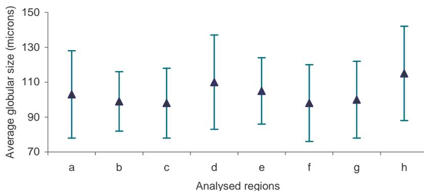
Figure 8 - Values of the average globular diameter in different regions of sample 200 x 200 mm; 0.8 mm thickness, thixocast at 634°C during 10 minutes.
