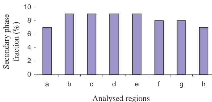
Figure 9 - Values of the secondary phase fraction in different regions of sample 200 x 200 mm; 0.8 mm thickness, thixocast at 634°C during 10 minutes.
