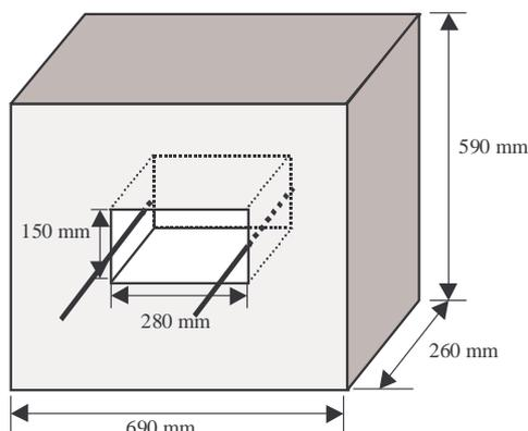
Figure 2 - Scheme of the furnace used in the preparation of thixocast sheets: dimensions 200 x 200 mm.
