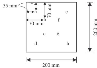
Figure 6 - Representative scheme of the regions of analysis of the thixocast sheet's microstructures, dimensions 200 x 200 mm.
