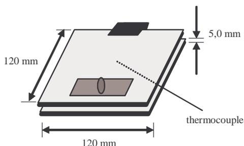
Figure 1 – Device used for the thermal treatments of controlled partial melting in samples of 100 x 100 mm.
