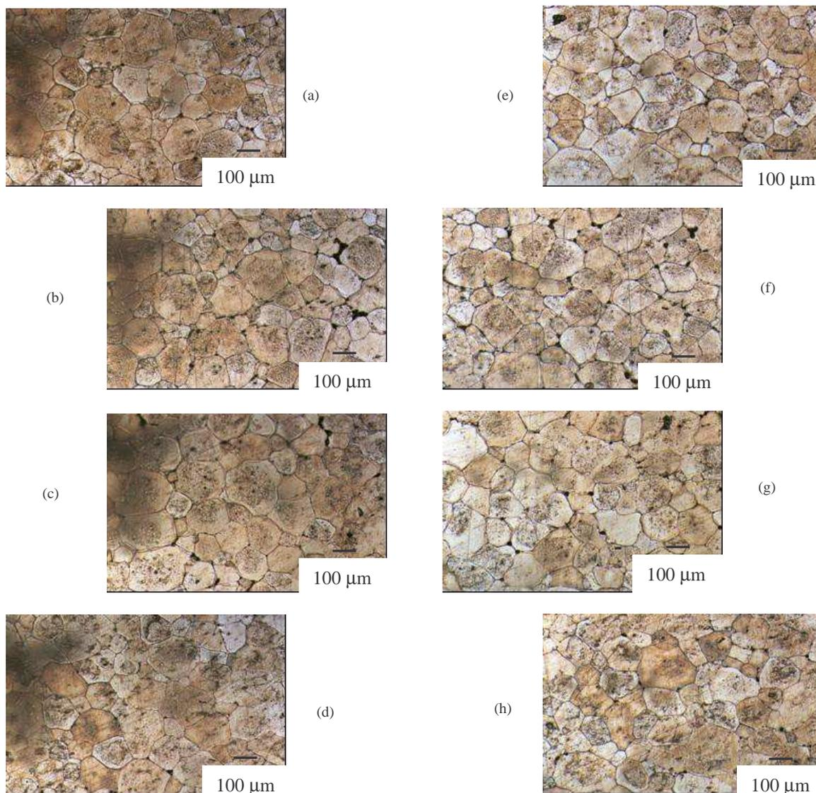
Figure 10 – Typical microstructures of a A5052 aluminium alloy sheet, 2.0 mm thickness, treated at 624°C during 5 minutes, in different regions. Sample with dimensions 200 x 200 mm, (a-h) regions of analysis.
