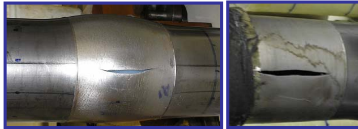
Figure 18. Details of the rupture zones for the machined and repaired pipes
