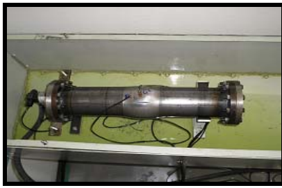
Figure 13. Machined pipe after burst
