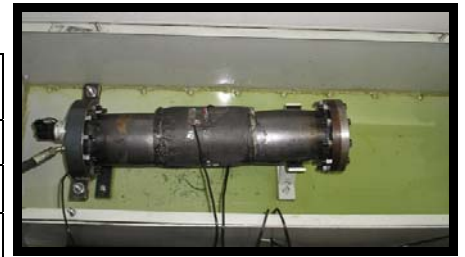
Figure 14. Repaired pipe after burst
