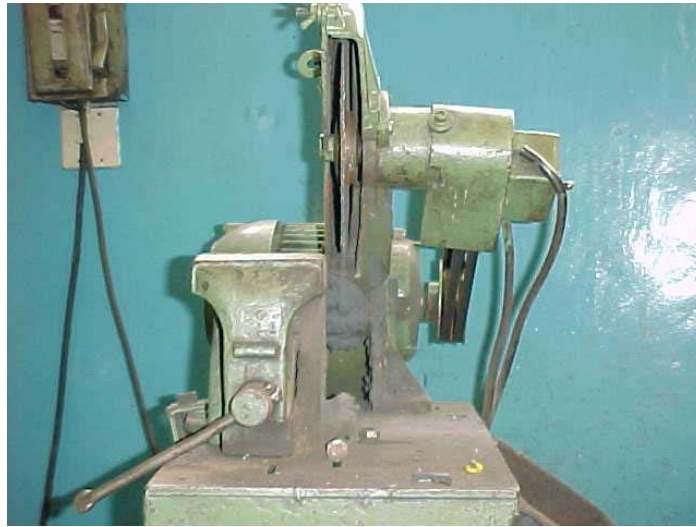
Figure 2. OP-10 – Device for cutting operation.
