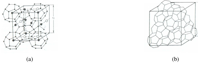
Figure 1 The classical hydrates formation structures, (a) structure I-type and (b) structure II-type.
