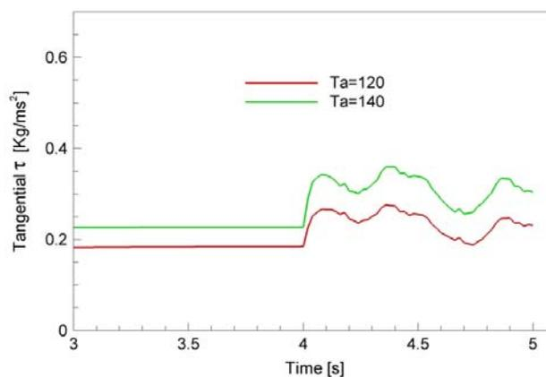
Figure 7. Temporal distribution of tangential shear stress, signal of numerical probe localized at  $r = 0.2$ ,  $\theta = 90^\circ$  and  $z = 0.3$ .
