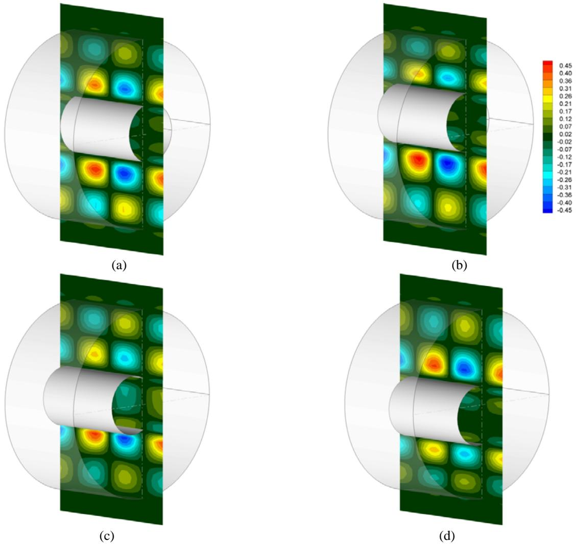
Figure 5. Instantaneous axial velocity field at  $Ta = 100$ ; (a)  $\alpha = 0^\circ$ , (b)  $\alpha = 72^\circ$ , (c)  $\alpha = 180^\circ$ , (d)  $\alpha = 252^\circ$ .
