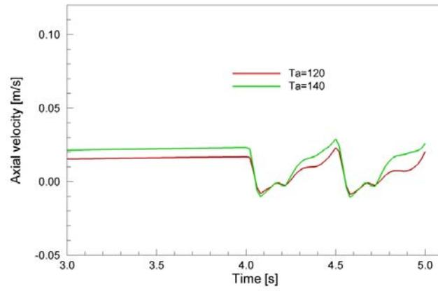
Figure 4. Temporal axial velocity distribution at the center point of the gap.
