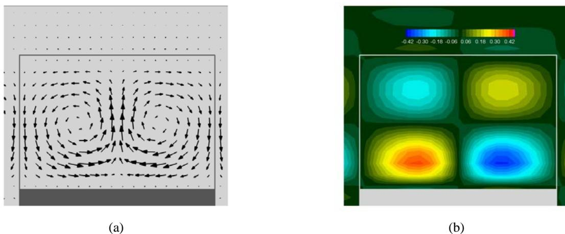
Figure 3. Taylor-Couette Flow at  $Ta = 100$ ; (a) Taylor vortices, (b) axial velocity component.
