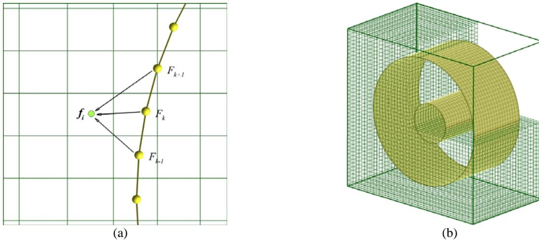
Figure 2. (a) Two-dimensional sketch of Lagrangian force distribution, (b) Eulerian and Lagrangian domain.
