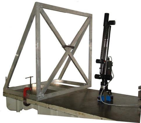
Figure 9 - Experimental construction with gauge, support and CMA
