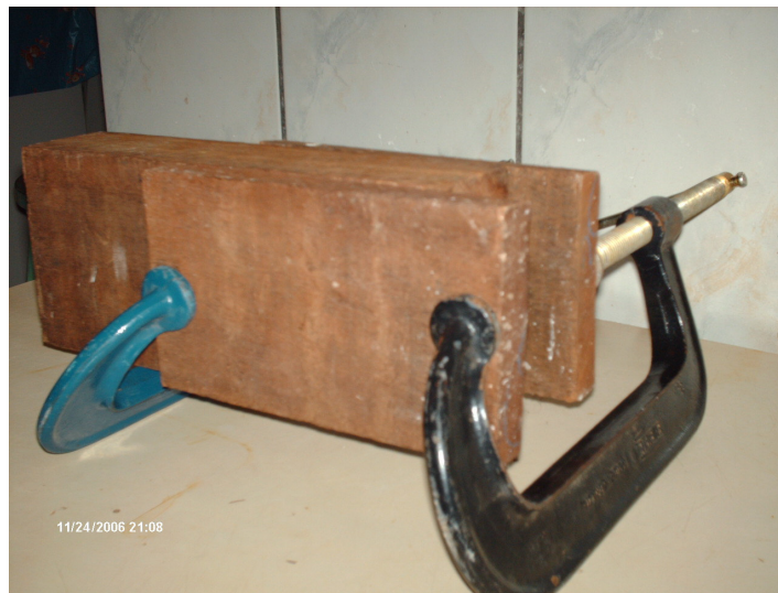
Figure 2. Assembly for testing bolted joint parallel to grain in compression.
