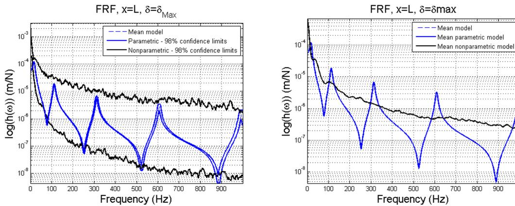
Figure 7. Mean model FRF with probability level of 98%, confidence region for both parametric and nonparametric probabilistic approach with maxima values of the coefficients of dispersion:  $\delta_{K_t} = 0.58$  and  $\delta_{[K]} = 0.96$  (left) and expected values for the FRFs, with maxima values of the coefficients of dispersion:  $\delta_{K_t} = 0.58$  and  $\delta_{[K]} = 0.96$  (right).
