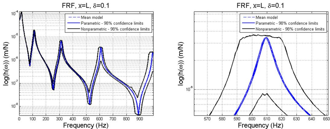
Figure 5. FRF of the mean model with probability level of 98%, for both parametric and nonparametric probabilistic approaches, taking  $\delta_{K_t} = \delta_{[K]} = 0.1$  (left). Zoom image (right).
