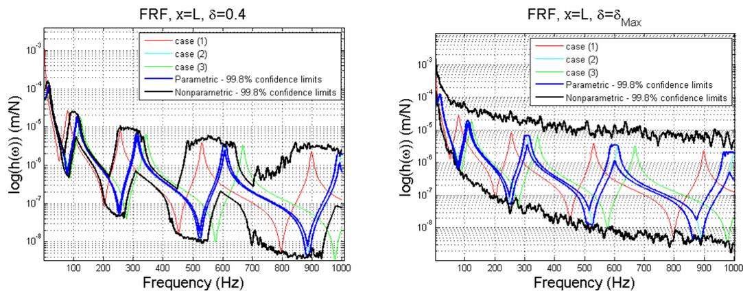
Figure 9. FRFs for three deterministic cases:  $\underline{K}_t = 0$ , clamped-free and clamped-locked, FRF for parametric and nonparametric approaches with probability level of 99.8%.  $\delta_{K_t} = \delta_{[\mathbf{K}]} = 0.4$  (left) and maxima values  $\delta_{K_t} = 0.58$  and  $\delta_{[\mathbf{K}]} = 0.96$  (right).
