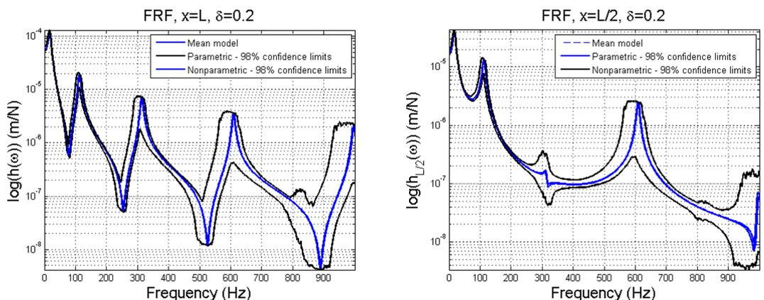
Figure 6. Mean model responses and confidence region for both parametric and nonparametric probabilistic approaches, taking  $\delta_{K_t} = \delta_{[K]} = 0.2$ : response at  $x = L$  (left) and response at  $x = L/2$  (right).
