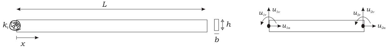
Figure 1. Beam modeled (left) and beam element (right).
